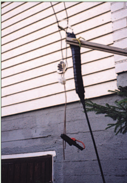
● During the setting-up phase crocodile clips are used to make the connections.
